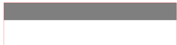
Fig. 2. Cross section view of a 100 \mu\text{m} thick slab detector volume (in grey) inserted at the top of the silicon die surface (red box).
