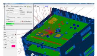
*Fig. 2. Screen shot of the electron tracks during reverse Monte Carlo calculation on an electronic equipment.*
