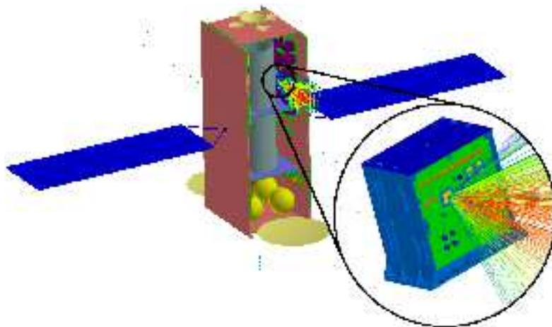
Figure 3 : FASTRAD Approach ; satellite and equipment (EREMS company courtesy) modeling
