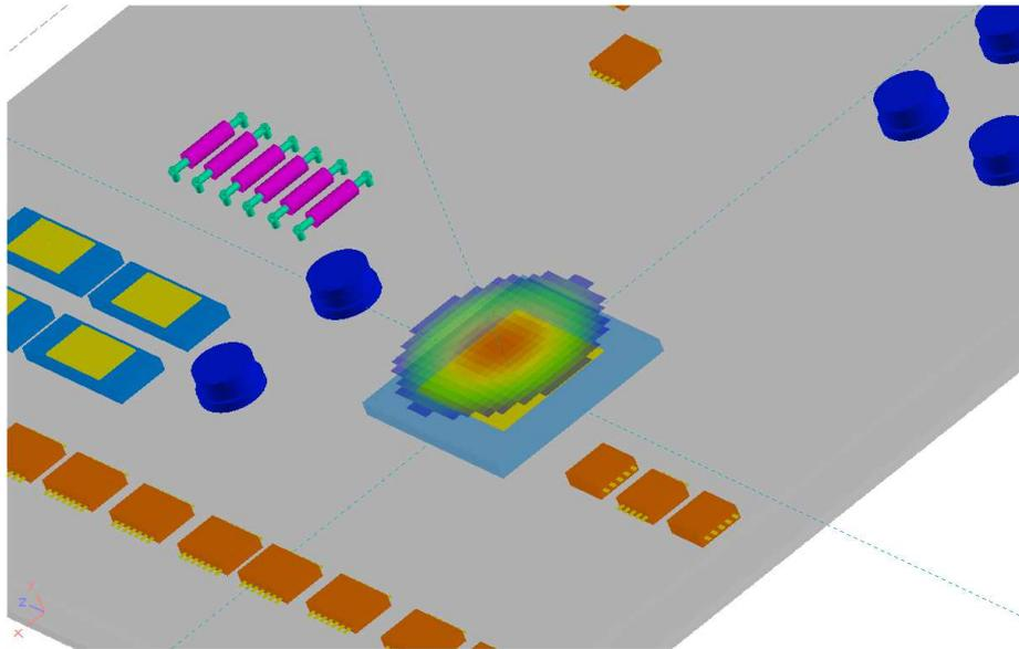
Figure 2 : Screenshot of the FASTRAD tool during a complete satellite analysis (CNES courtesy)
