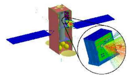
Figure 3 : FASTRAD Approach ; satellite and equipment (EREMS company courtesy) modeling
