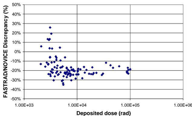
Fig. 8. FASTRAD/NOVICE discrepancy according to the deposited dose in FASTRAD for trapped (blue line) electrons.
