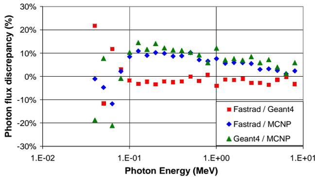
Fig. 5, Ratio between transmitted photon numbers in the sphere detector for a 10MeV electron beam: FASTRAD to MCNPX (blue diamond), FASTRAD to GEANT4 (red square), and GEANT4 to MCNPX (green triangle).
