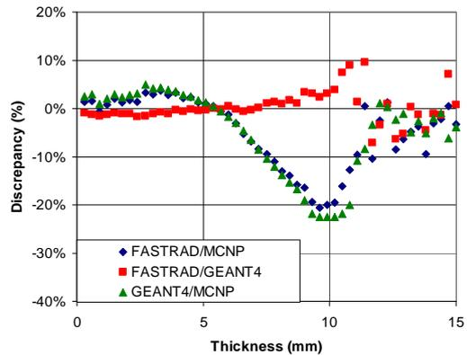
Fig. 3, Ratio between deposited dose from FMC tools in Aluminum layers according to the crossed thickness: FASTRAD to MCNPX (blue diamond), FASTRAD to GEANT4 (red square), and GEANT4 to MCNPX (green triangle).
