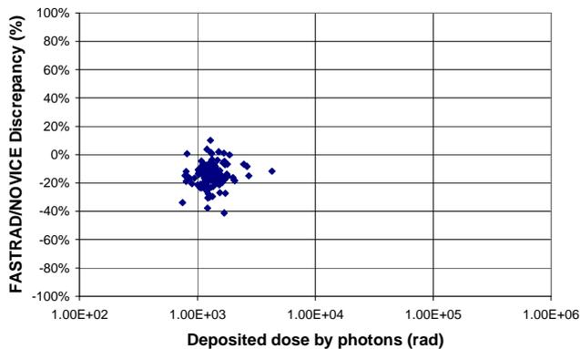
Fig. 10, FASTRAD/NOVICE discrepancy according to the deposited dose in FASTRAD for trapped (blue line) electrons, only considering the transmitted photons.
