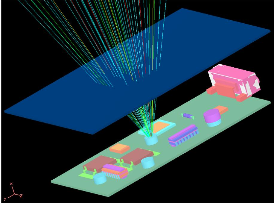
Fig. 3. Post processing of a ray tracing calculation.
