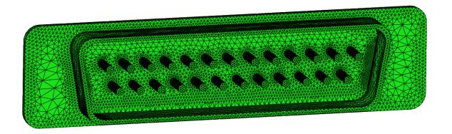
• Several conductivity models are available: radiation-induced conductivity, temperature and electric field dependant conductivity, constant conductivity, user defined electric field-induced conductivity
